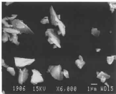
Figure 1.27 Scanning electron microscope picture of fine fraction of ground silicon: typical particle size 2–3 \mu\text{m} (Courtesy of W. C. Wedberg).
