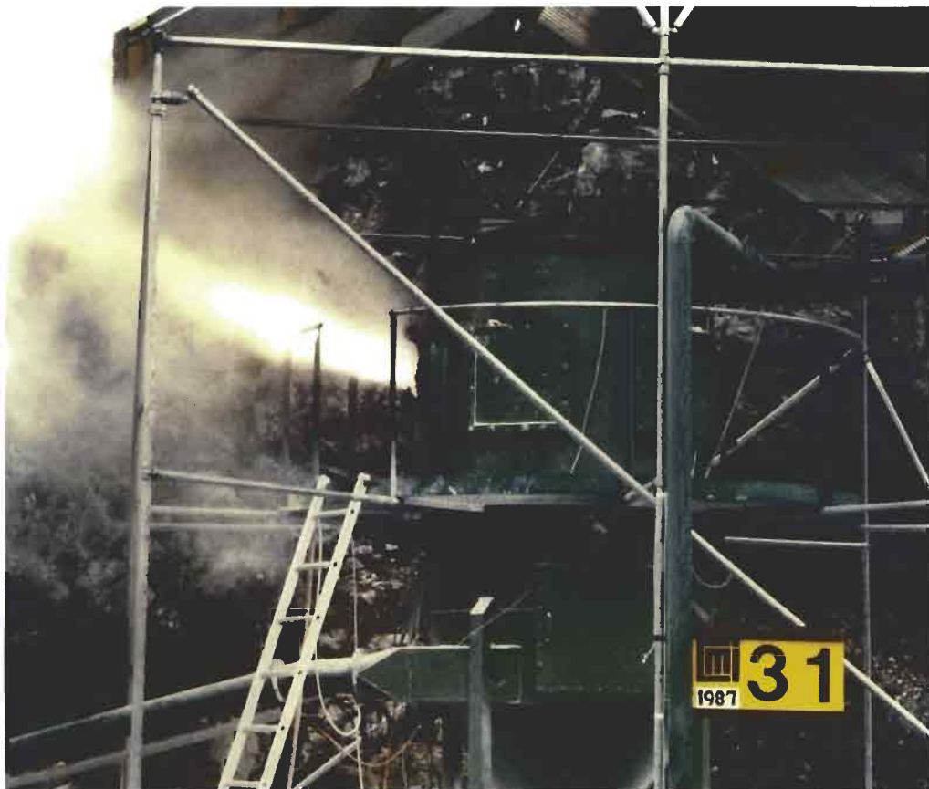
Plate 8 Maize starch explosion in 5.8 m 3 experimental bag filter unit in Norway. Vent area is 0.16 m 2 . Static opening pressure of vent cover is 0.10 bar(g). Maximum explosion pressure is 0.15 bar(g).
