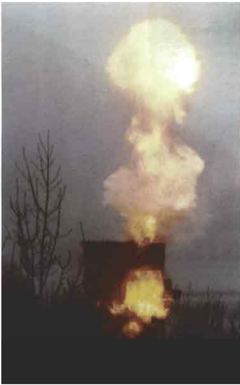
Plate 5 High-turbulence maize starch explosion in 500 m 3 bolted steel plate silo at Vaksdal, Norway, in April 1982 (Photographer: A. M. Fosse, Vaksdal).
