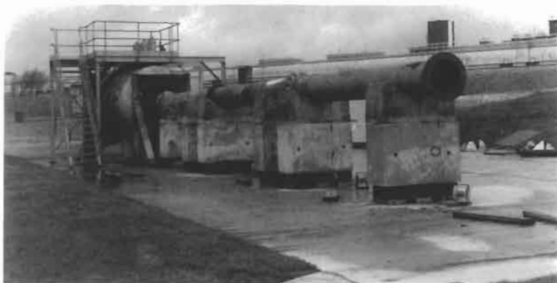
Figure 1.111 18.5 m 3 vented explosion vessel connected to a straight vent duct (Courtesy of Health and Safety Executive, United Kingdom). For a much clearer picture, see Color Plate 1.
