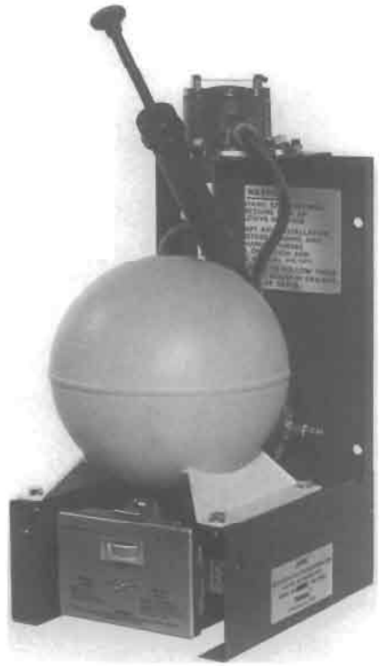
Figure 1.121 A self-contained automatic explosion suppression unit (X-PAS) consisting of a pressurized spherical suppressant container with an explosive charge-operated valve, a pressure detector, and a long-life lithium battery power unit (Courtesy of Fenwal Inc., Ashland, MA).
