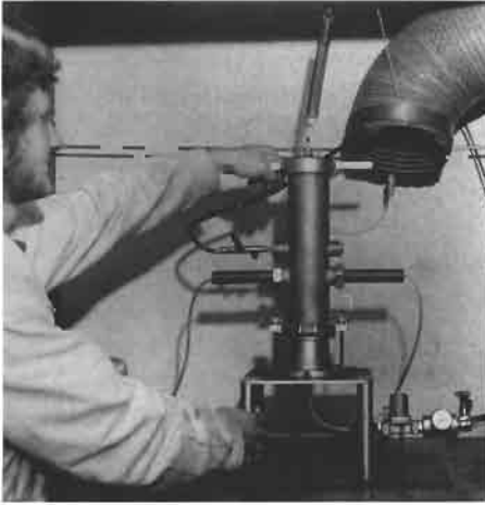
Figure 7.50 Photograph of the version of the Hartmann bomb shown in Figure 7.49.
