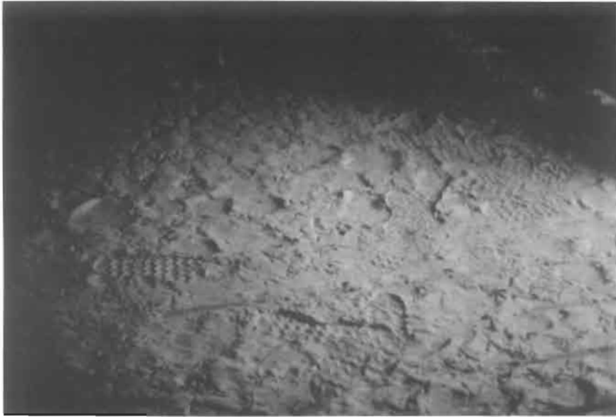
Figure 2.11 Dust accumulation on the floor in the head house of a grain silo plant in the United States (Courtesy of C. W. Kauffman, University of Michigan).
