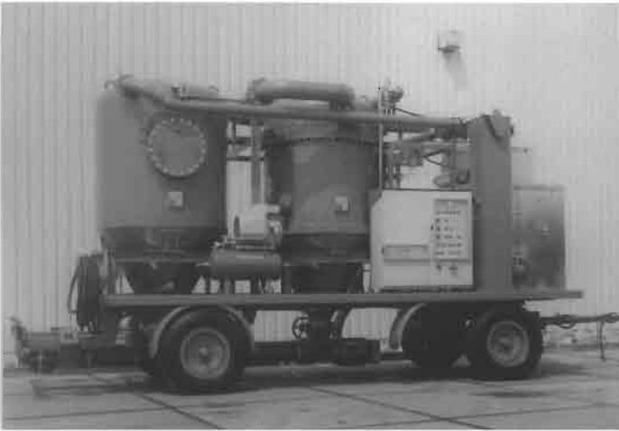
Figure 1.130 Large mobile vacuum cleaner for explosible dusts in industry. The vessels and connecting ducts are designed to withstand internal pressures of 9 bar(g). The power requirement is 45–55 kW (Courtesy of Edelhoff Polytechnik GmbH, Iserlohn, Germany).
