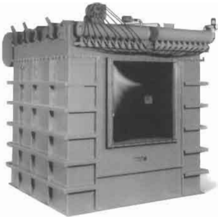
Figure 1.94 The basic principle of dust explosion venting: Provision of an opening controlled discharge of unburned, burning, and burned dust cloud keeps the maximum pressure inside the vessel below a predetermined limit, P_{red} .
