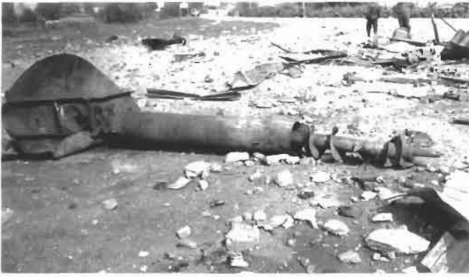
Figure 2.31 Top of 5.2 m 3 premix and 3.3 m long mixing screw with surrounding steel tube (see Figure 2.30), as found after the explosion 12 m away from location of the mixer prior to the explosion (Courtesy of E. Berg, Dyno Industries, Gullaug, Norway).
