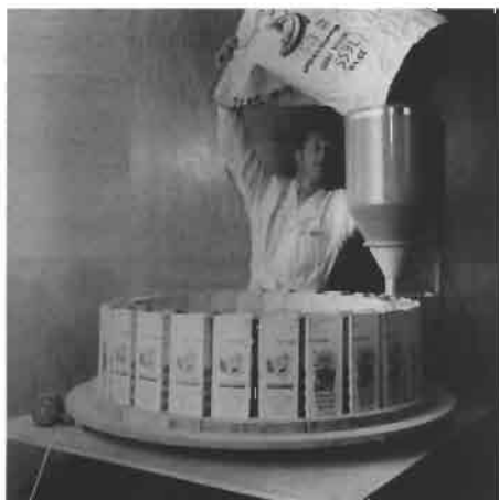
Figure 7.3 Large spinning riffler used at the Chr. Michelsen Institute, Norway, for splitting large natal samples of grain dust into 26 subsamples.
