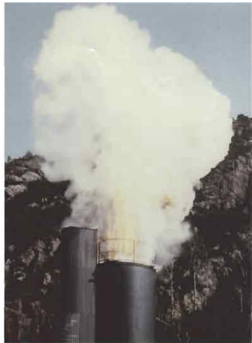
Plate 7 Vented maize starch explosion in 236 m 3 steel silo in Norway.
