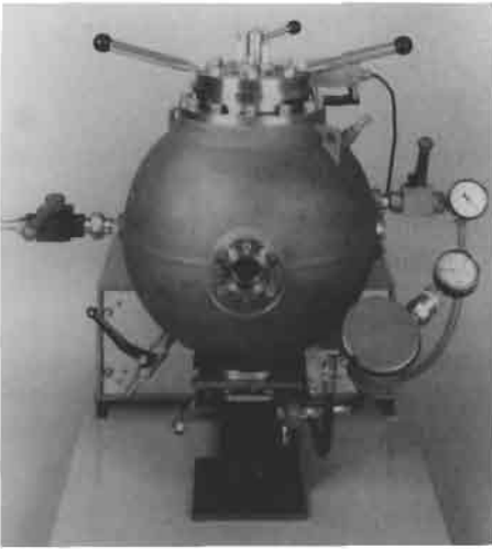
Figure 7.56 A 20 liter Siwek sphere to determine pressure development in dust explosions (Courtesy of R. Siwek, Cuba-Geigy AG, Switzerland).
