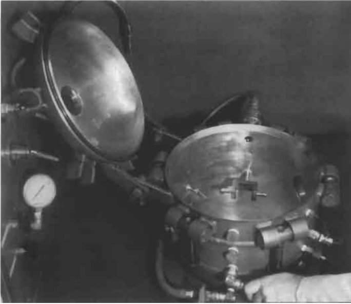
Figure 7.44 Photograph of opened 20 liter U.S. Bureau of Mines explosion vessel, showing one of the light attenuation probes for measuring dust concentration (Courtesy of K. L. Cashdollar, U.S. Bureau of Mines, Pittsburgh).
