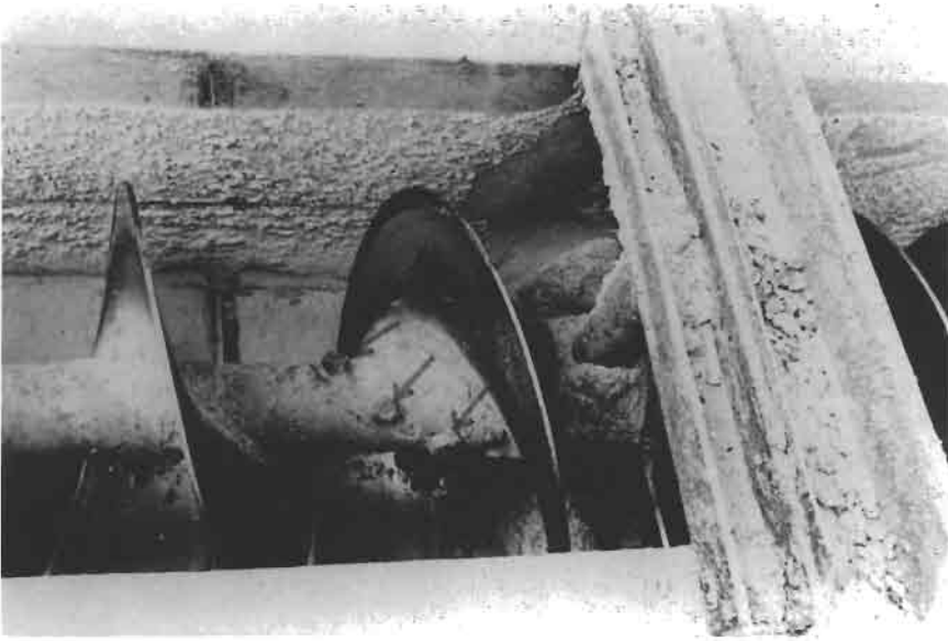
Figure 2.17 Part of a screw conveyor in the exploded fish meal plant showing fixing bolts.
