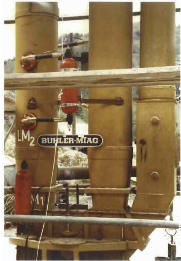
Plate 4 Application of automatic dust explosion suppression to bucket elevators (Courtesy of T. Pinkwasser, Bühler, Switzerland).
