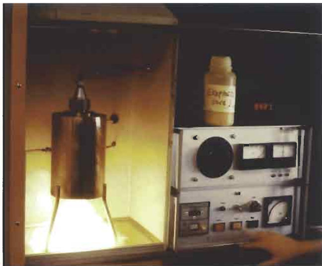
Plate 10 Ignition of a dust cloud in the Godbert-Greenwald furnace.
