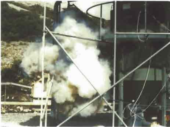
Plate 3 Venting of a polypropylene/air explosion in a 5.8 m 3 bag filter unit without (top) and with (bottom) quenching tube (Courtesy of F. Alfert and K. Fuhr, Chr. Michelsen Institute, Bergen, Norway).
