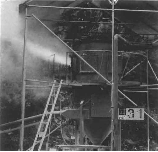
Figure 6.18 Maize starch explosion in a 5.8 \text{ m}^3 experimental bag filter unit in Norway. Vent area is 0.16 \text{ m}^2 . Static opening pressure of the vent cover is 0.10 \text{ bar(g)} . Maximum explosion pressure is 0.15 \text{ bar(g)} . For a much clearer picture, see Color Plate 8.
