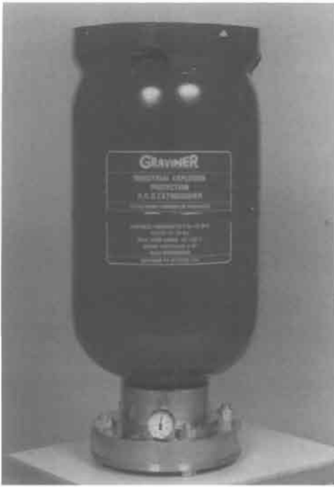
Figure 1.120 Large 45 liter high-rate suppressor for very fast discharge of 35 kg of MH_4H_2PO_4 powder. The diameter of the explosive charge-operated valve is 127 mm (5 in.) and the driving gas is nitrogen at 60 bar (Courtesy of Kidde-Graviner, Colnbrock, United Kingdom).
