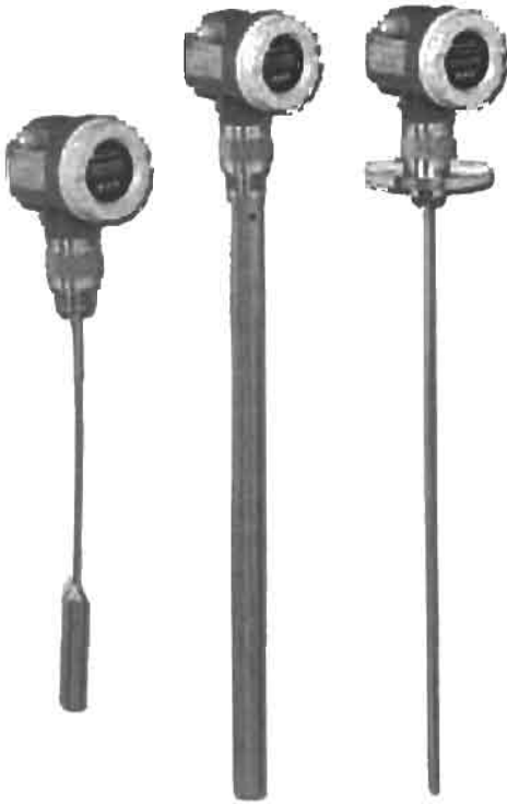
Figure 8.7 Three models of a capacitive surface level indicator. The model to the left, with a metal rope carrying a weight at the end, is for powders and granulates in silos. The two other models, with coaxial and plain metal rods respectively, are for liquids in tanks (Courtesy of G. Klotz-Engmann, Endress + Hauser, Germany).
