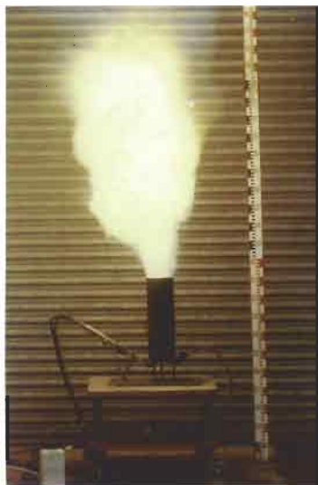
Plate 9 Silicon dust explosion in the welding torch ignition test apparatus used in Norway.
