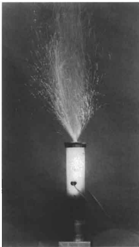
Figure 7.35 Silicon dust explosion following electric spark ignition in an apparatus of the type illustrated in Figure 7.34.
