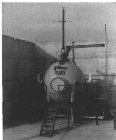
Figure 7.63 A 10 m 3 test vessel for assessing the efficacy of suppression systems for volumes larger than 1 m 3 (Courtesy of Fike Corporation, United States).
